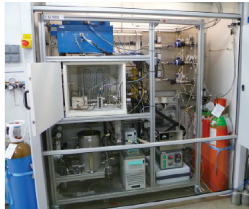
IFPEN – Pilot unit for CO 2 electroreduction
